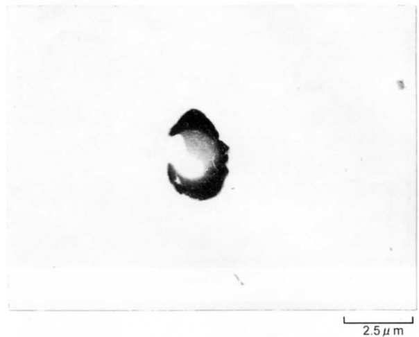
Fig. 10 FE-SEM photomicrograph of sphere graphite with inclusion. This sphere graphite was observed at a different area from that analyzed by CMA in the same chilled sample.
